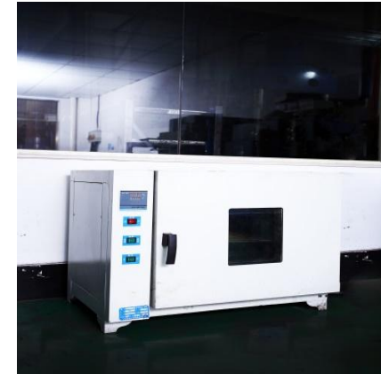
Electric Thermostat Box
