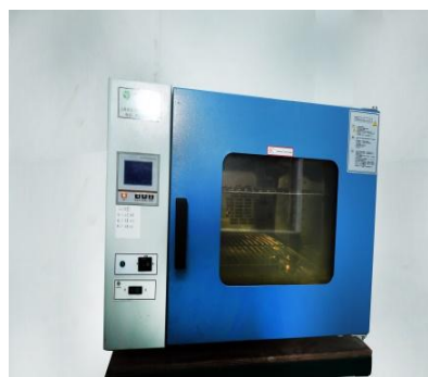
High Temperature Test Chamber
